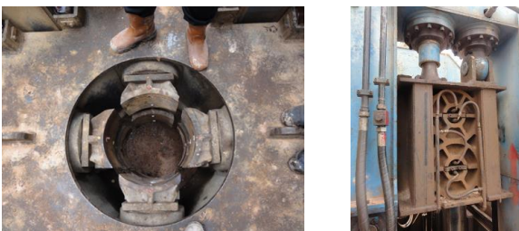
Figure 3 Hydraulic gripping system with gripping blocks
