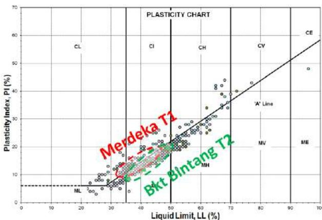
Figure 3D Plasticity Chart of Kenny Hill Soils
