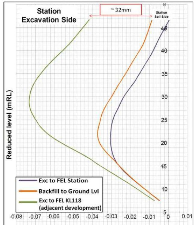
Figure 10 Merdeka Station - Analysed displacement Envelopes
