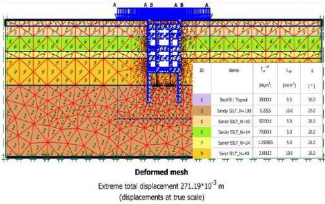
Figure 11 Bukit Bintang Station - Plaxis Meshing Model
