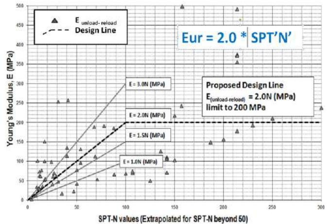
Figure 6  $E_{ur}$  versus SPT 'N' plot of Kenny Hill Soils
