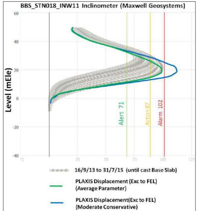
Figure 18 Displacement profiles from Inclinator INW11 Bukit Bintang T2 D-wall panel, taken from the project online data management system Maxwell geosystems' Mission OS Portal
