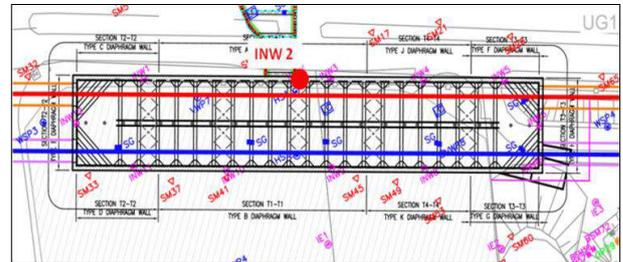
Figure 14 Merdeka in-wall Inclometer INW2 for T1 D-wall
