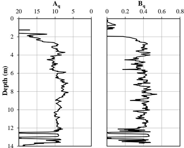
Figure 15 Profiles of  $A_q$  and  $B_q$  derived from the piezocone test shown on Figure 3
