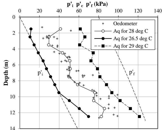
Figure 19 Profiles of  $p'_c$  derived from piezocone test parameter  $A_q$  but investigating the effect of cone preparation temperature
