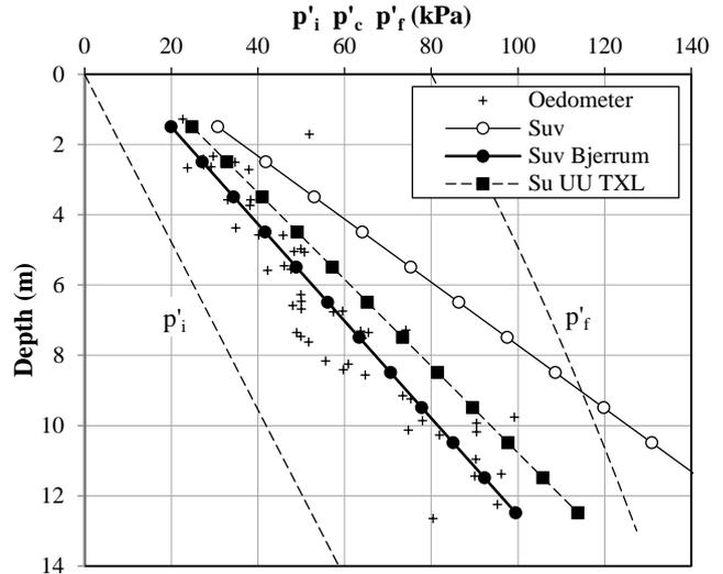
Figure 14 Profiles of  $p'_c$  derived from undrained shear strength following three different assessments
