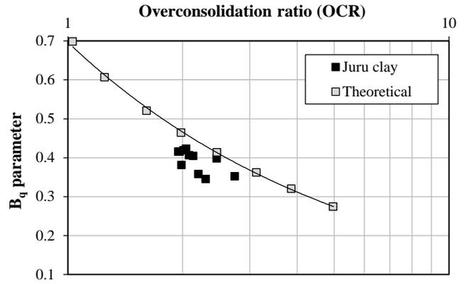
Figure 16 Relationship between OCR and  $B_q$  according to Wroth (1988) including data from the Juru site
