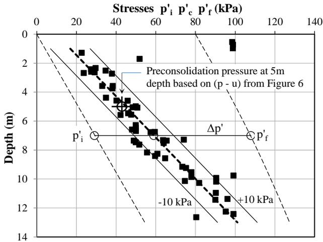
Figure 8 Stresses which control the settlement calculation
