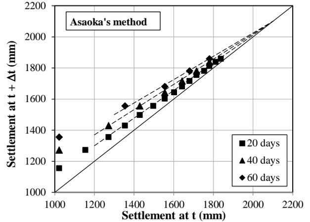
Figure 7 Assessment of final settlement of embankment with drains using Asaoka's method
