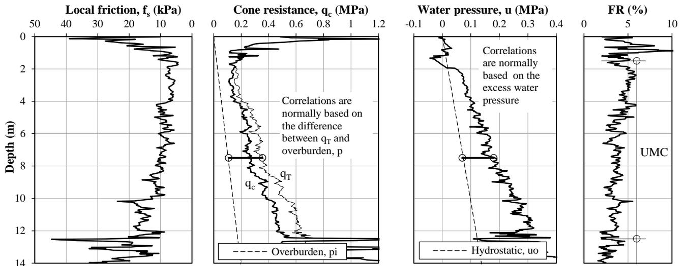
Figure 3 Typical piezocone (CPTu) profile through the Holocene marine clay at Juru
