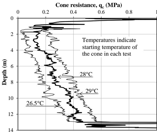
Figure 18 Profiles of  $q_c$  measured at the Juru site affected by the preparation temperature of the cone
