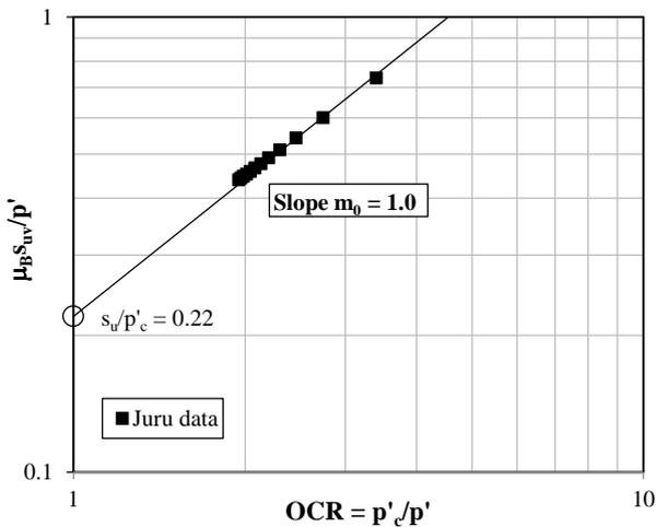
Figure 13 Independence of  $s_{uv}/p'_c$  from OCR, based on oedometer and corrected vane test data for the Juru site, after Mesri et al (1994)
