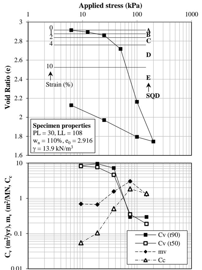
Figure 9 Oedometer consolidation test on specimen from 5.5m
