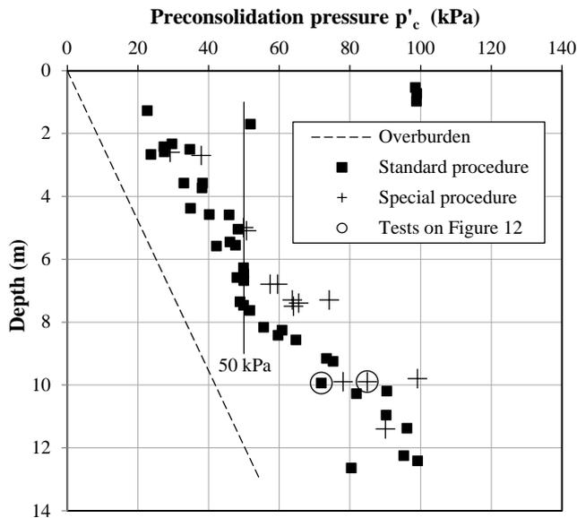
Figure 10 Profile of preconsolidation pressure at Juru based on oedometer consolidation tests
