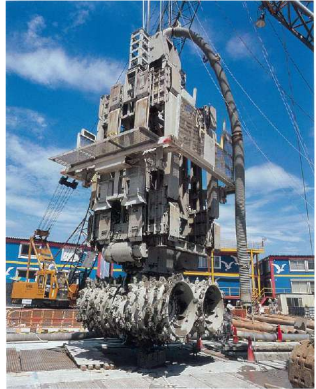
Figure 49 Two-axes rotating type cutting bits
