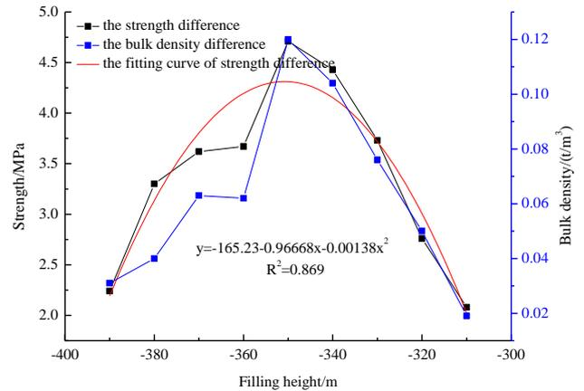
Figure 6 The strength difference and bulk density difference at 100m stage
