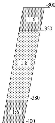
Figure 12 Design value of 100m segment with high stage cemented backfill
