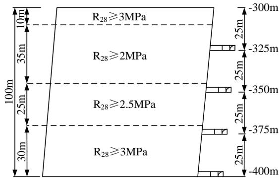
Figure 1 The first-step filling strength distribution of the high stage stope
