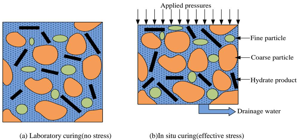
Figure 7 Schematic representation of the effect of curing stress
