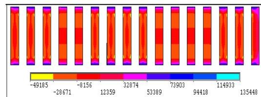
Figure 11 Tensile stress of 1:8 cemented backfill
