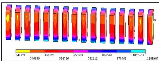
Figure 8 Compressive stress of 1:4 cemented backfill
