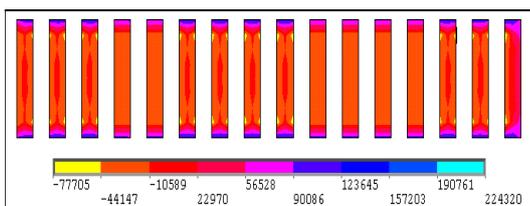
Figure 9 Tensile stress of 1:4 cemented backfill
