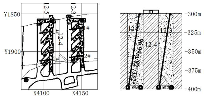
Figure 3 The coring arrangement of 12-3# and 12-5# stope
