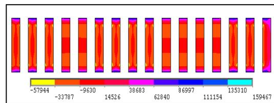
Figure 10 Tensile stress of 1:6 cemented backfill
