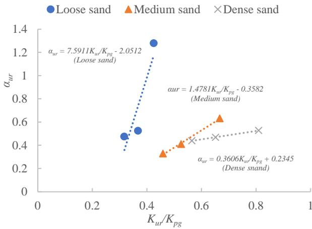
Figure 8  $\alpha_{ur}$  versus  $(K_{ur}/K_{pg})$  for loose, medium, and dense sand
