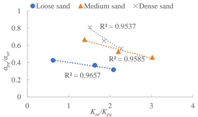
Figure 5 ( $\alpha_{pg}/\alpha_{ur}$ ) versus ( $K_{ur}/K_{pg}$ ) for loose, medium, and dense sand
