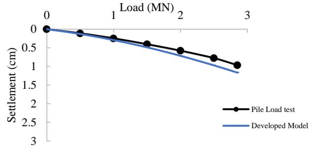
Figure 2 Load–Settlement Curves for pile load test and developed model
