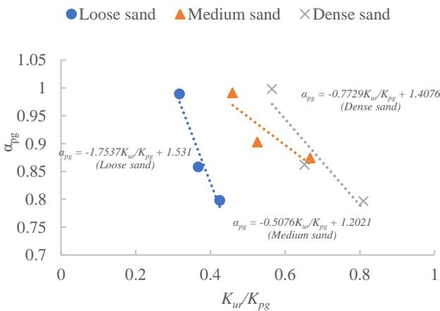
Figure 9  $\alpha_{pg}$  versus  $(K_{ur}/K_{pg})$  for loose, medium, and dense sand
