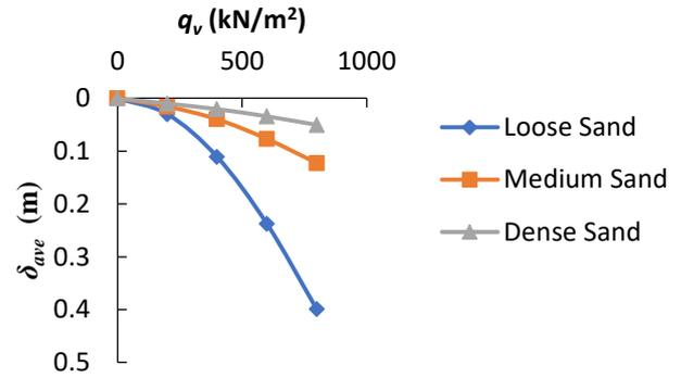
Figure 6  $q_v-\delta_{ave}$  of piled raft of  $S = 7D$  for different sand conditions
