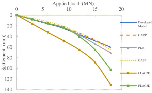
Figure 3 Load-settlement curves of piled raft model
