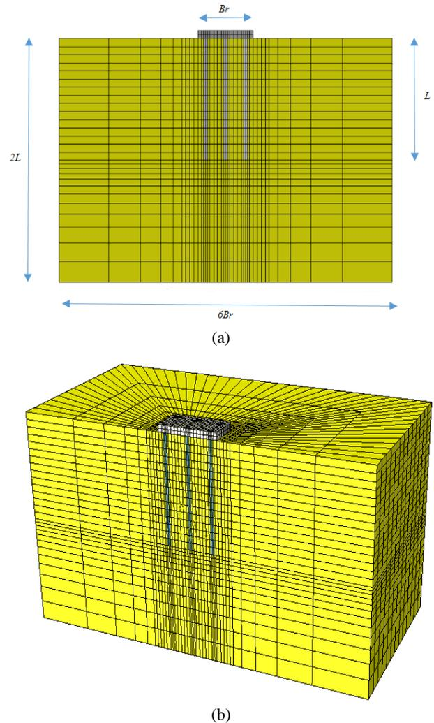
Figure 1 (a) Elevation view of finite element mesh, (b) one half symmetry view of pile raft models
