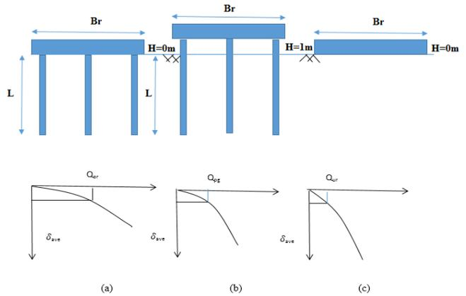
Figure 4 Typical configuration and load–settlement curves of (a) piled raft (b) pile group (c) unpiled raft
