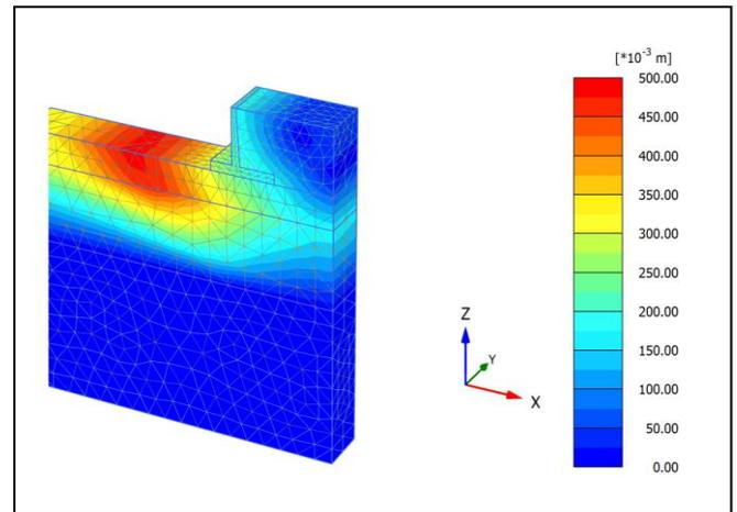
Figure 5 Total Displacement Distribution in (m) Resulting from Swelling of Expansive Soil for Unpiled Case
