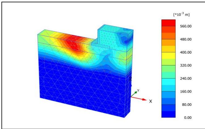
Figure 17 Total Displacement Distribution in (m) of Cantilever Wall Retaining Resulting from Swelling in Expansive Soil for Three Vertical and Three Horizontal Helical Piles under the Base and Beside Wall of Retaining Wall (L/H=3.2)
