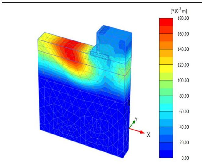
Figure 14 Total Displacement Distribution in (m) Resulting from Swelling of Expansive Soil of Cantilever Retaining Wall for Two Vertical and One Inclined Helical Piles under the Base of Retaining Wall (L/H=3.2)
