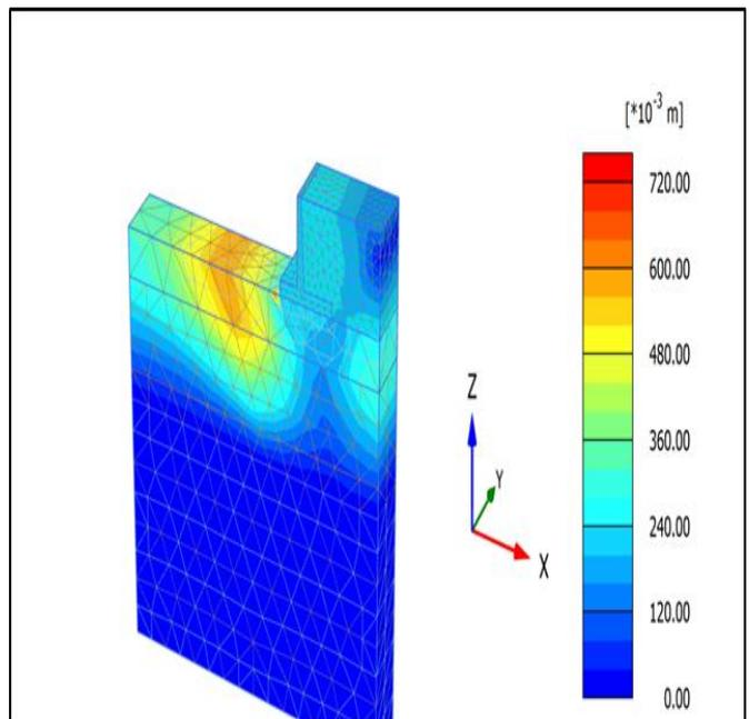
Figure 11 Total Displacement Distribution in (m) Resulting from Swelling in Expansive Soil of Cantilever Retaining Wall for Three Vertical Helical Piles under the Base of Retaining Wall (L/H=3.2)
