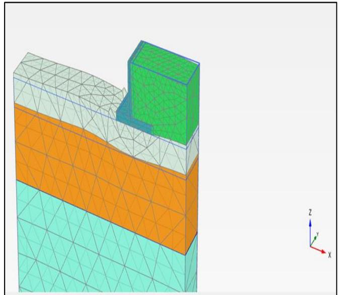
Figure 10 Deformed Shape of Cantilever Retaining Wall after Swelling of Expansive Soil for Three Vertical Helical Piles under the Base of Retaining Wall (L/H=3.2)
