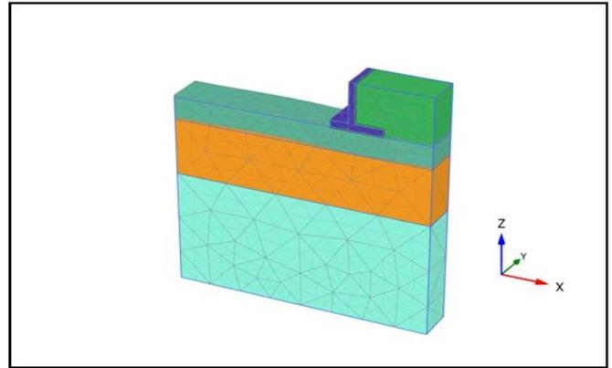
Figure 4 Deformed Shape of Cantilever Retaining Wall after Swelling of Expansive Soil for Unpiled Case
