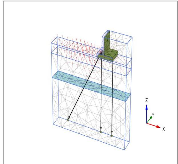
Figure 15 Vectors of Total Displacement of Cantilever Retaining Wall Resulting from Swelling of Expansive Soil for Two Vertical and One Inclined Helical Piles under the Base of Retaining Wall (L/H=3.2)
