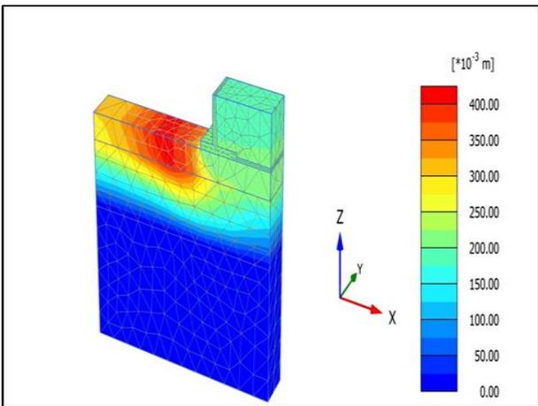
Figure 8 Total Displacement Distribution in (m) of Cantilever Retaining Wall Resulting from Swelling in Expansive Soil for Two Vertical Helical Piles under the Base of Retaining Wall (L/H=2)
