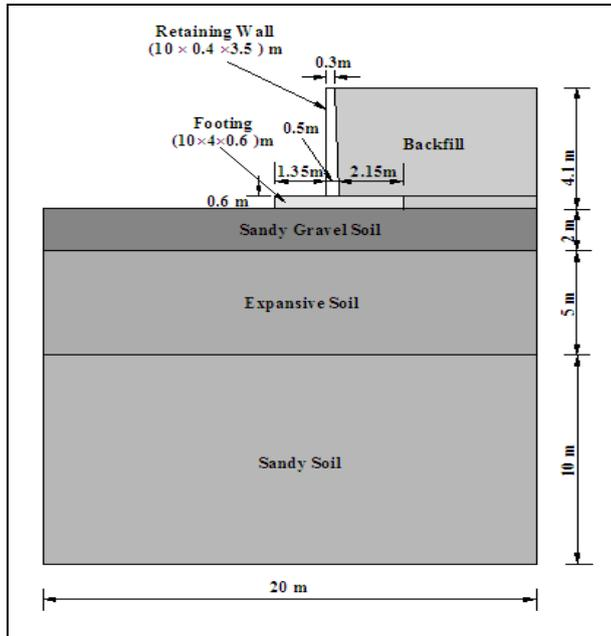
Figure 2 Cantilever Retaining Wall Problem
