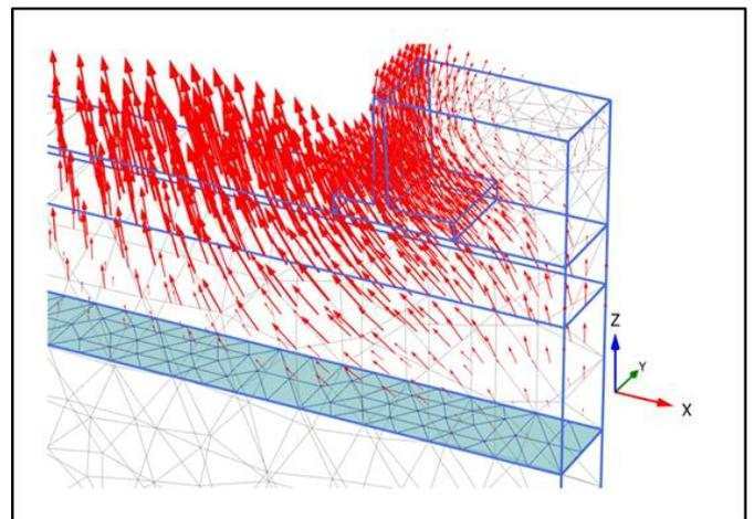
Figure 6 Vectors of Total Displacement Resulting from Swelling of Expansive Soil for Unpiled Case.
