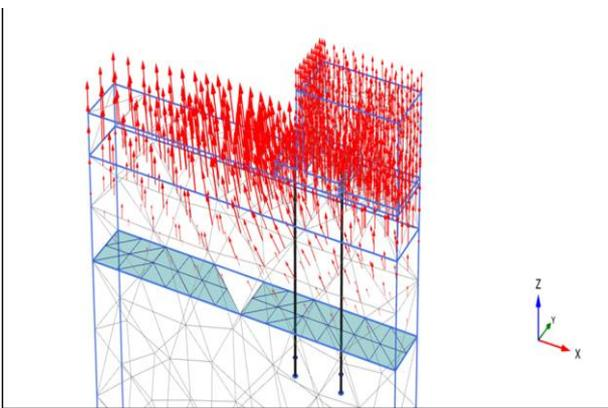
Figure 9 Vectors Total Displacement of Cantilever Retaining Wall Resulting from Swelling of Expansive Soil for Two Vertical Helical Piles under the Base of Retaining Wall (L/H=2)
