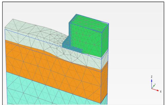
Figure 16 Deformed Shape of Cantilever Retaining Wall after Swelling of Expansive Soil for Three Vertical and Three Horizontal Helical Piles under the Base and Beside Wall of Retaining Wall (L/H=3.2)
