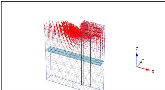
Figure 18 Vectors of Total Displacement Distribution of Cantilever Retaining Wall Resulting from Swelling in Expansive Soil for Three Vertical and Three Horizontal Helical Piles below Base and Beside Wall of Retaining Wall (L/H=3.2)
