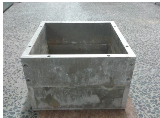
Figure 3 Durability split mould for easier demoulding after shearing (After Oderah, 2015)
