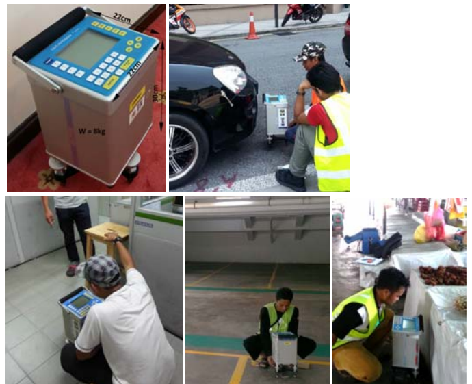
Figure 5a Typical gravity meter (CG-5), 5b Operation along car parking bay, 5c Operation within the office, 5d Operation at the building basement, 5e Operation within a food market
