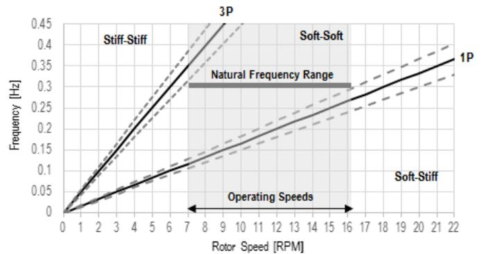
Figure 6 Campbell diagram for natural frequency design range (Von der Haar, 2014)
