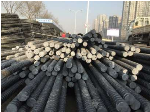
Figure 5 GFRP Reinforcements of Piles
