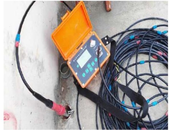
Figure 10 Readout Probe for Deflection Measurement of Pile
