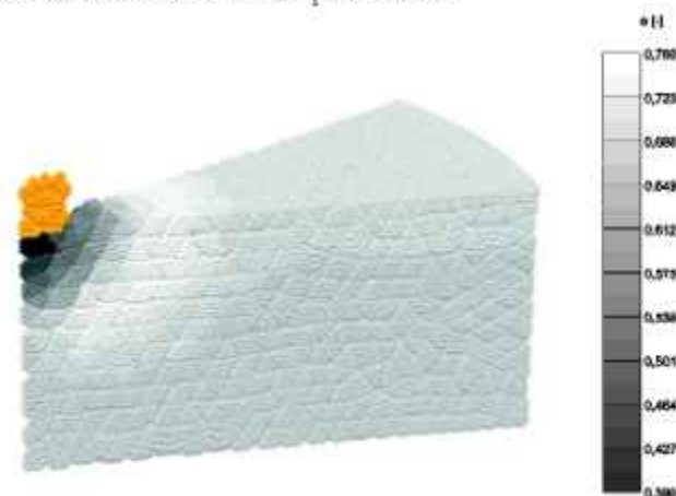
Figure 10 Void ratio distribution after one impact
