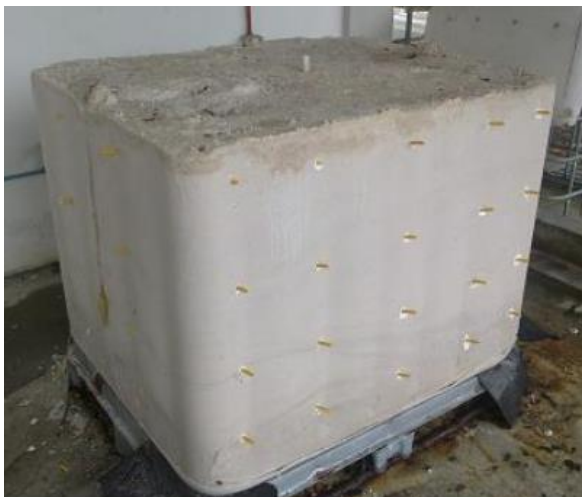
Figure 2 Photo of 1 m 3 sand block after treatment
