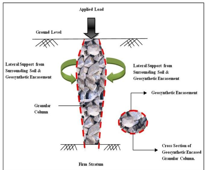
Figure 3 Single Encased Granular Column - Schematic Representation
