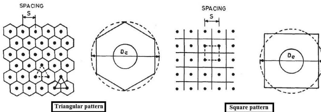
Figure 1 Various patterns of Stone Column Arrangement
