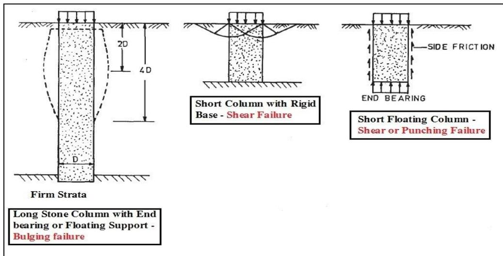
Figure 2 Failure Mechanisms of a Single Stone column
