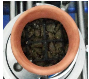
Figure 1 (b): Geogrid sample prepared
