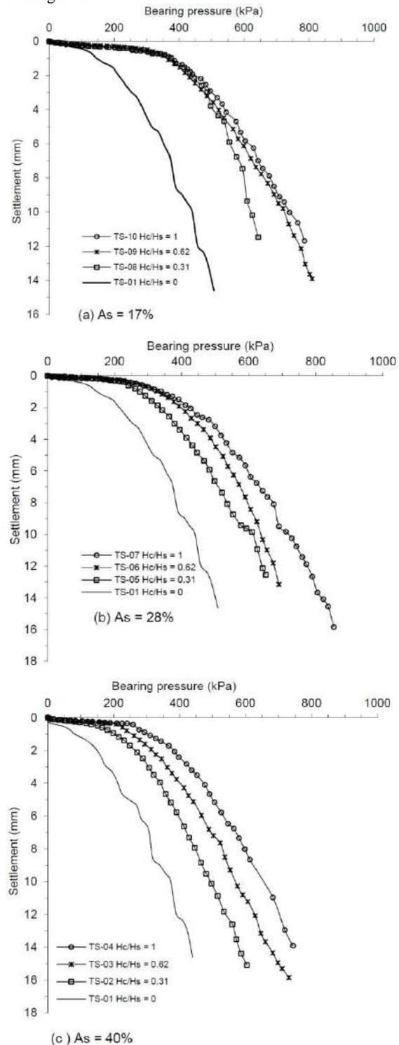
Figure 9 Displacement-bearing pressure for three area displacement ratio
