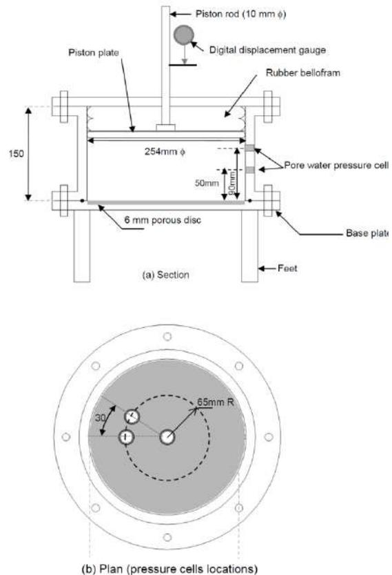
Figure 18 Schematic of one dimensional testing chamber
