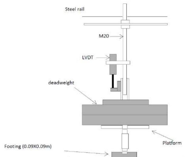
Figure 21 Foundation loading
