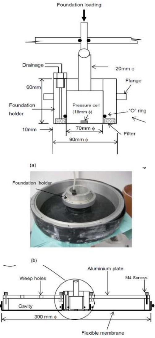
Figure 12 Footing and testing conditions away from footing
