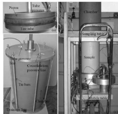
Figure 8 Sample preparation in one-dimensional consolidation chamber
