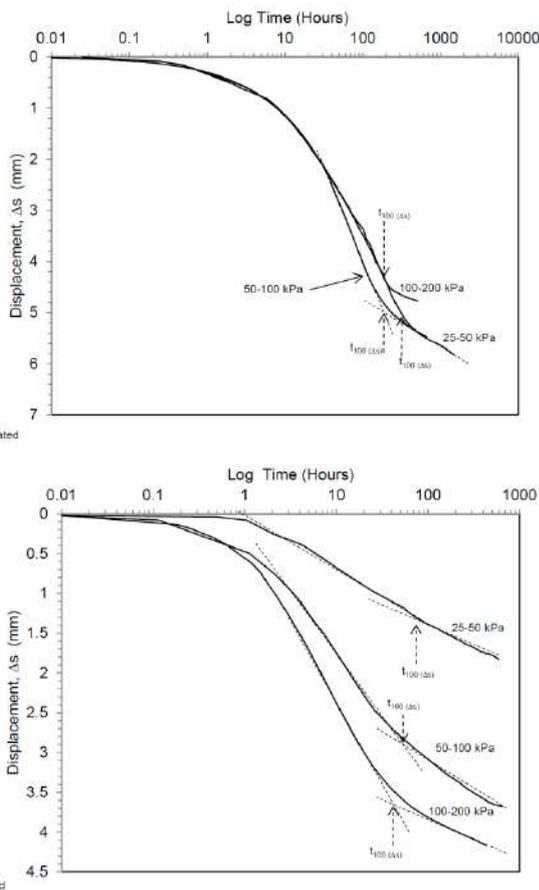
Figure 19 Settlement versus logarithm of time for sleetch with and without granular column
