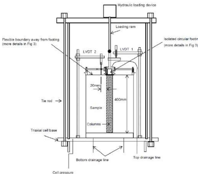
Figure 11 Testing chamber for assessing settlement of footing supported on circular footing under realistic boundary conditions
