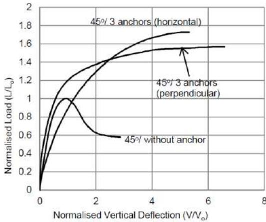
(a) Effects of horizontal and perpendicular columns
