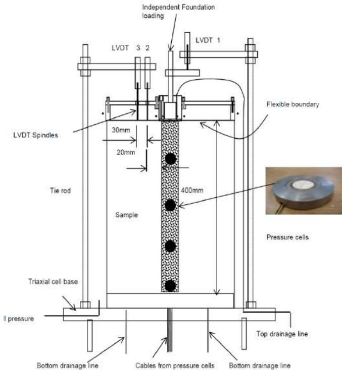
Figure 15 Assembled sample
