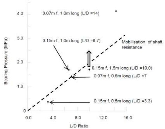
Figure 25 Bearing pressure vs L/D ratio QUB site
