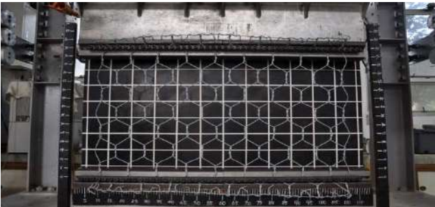
Figure 2 Schematic view of wire mesh panel tensile test setup
