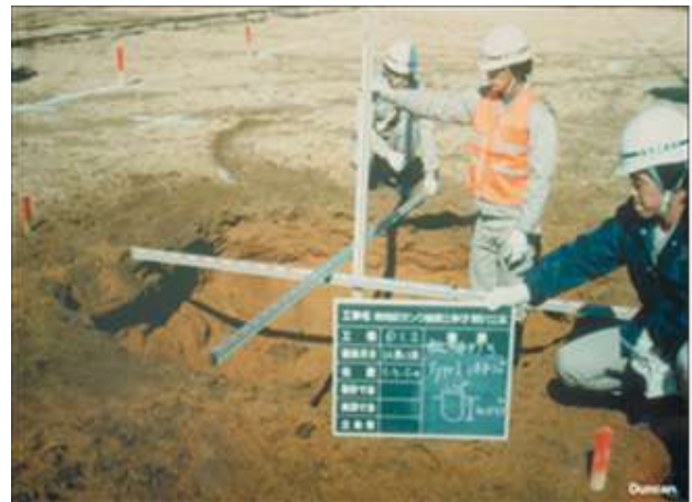
Figure 13 Measurement of Crater Volume
