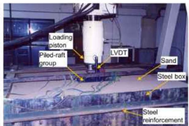
Figure 3 Laboratory tests setup: (a) General setup; (b) Installation of 2x2 group piled-raft; (c) Installation of 3x3 group piled-raft; (d) Raft installation of 3x3 group piled-raft with load cells; (e) Load application process
