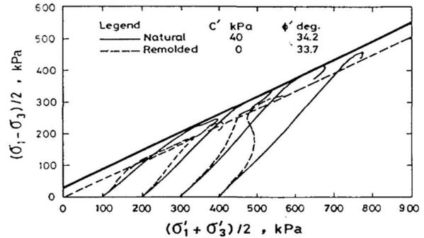
Figure 3 Effective stress path and failure envelope for naturally cemented and remolded specimens, Depth = 0.3 m (Ismael, 1999)
