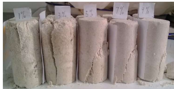
Figure 4 Specimen failure model of S-L mixed soil
