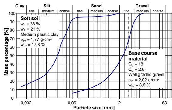
Figure 2 Soft soil and base course material used in the model scaled loading tests
