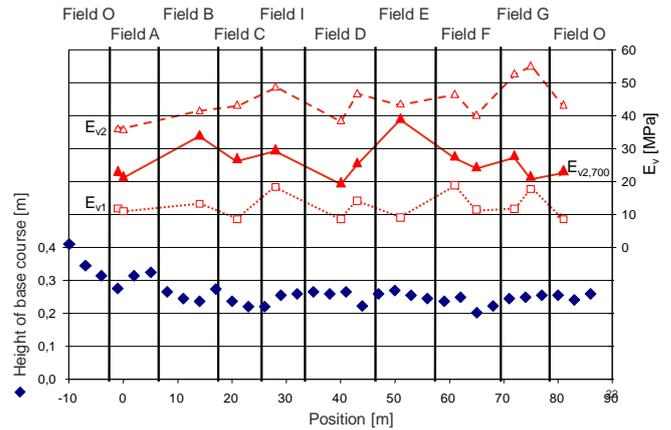
Figure 17 Thickness of base course layer (right side ordinate) and test results from static plate load tests  $E_{v1}$  and  $E_{v2}$  (left side ordinate) according to ASTM D1194/1195/1196 (German DIN 18134); modified static plate loading test up to 700 kPa mean stress evaluated by the modulus  $E_{v2,700}$
