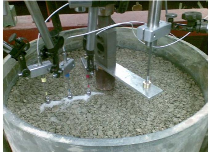
Figure 3 Loading on top the surface of the base course
