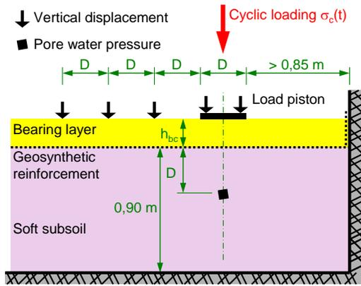
Figure 7 Large scale static and cyclic loading tests
