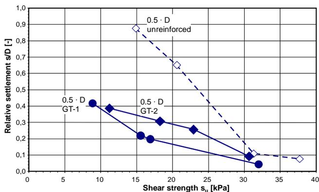
Figure 6 Settlement  $s/D$  of the model footing after 100000 cycles at a base course thickness of 0.5 D
