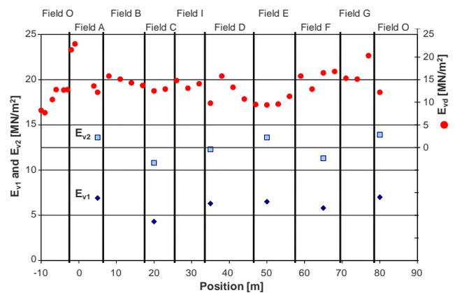
Figure 16 Tests results from static (modulus first loading  $E_{v1}$  and modulus reloading  $E_{v2}$ ) according to German DIN 18134 and ASTM D1194/1195/1196 respectively as well as results from dynamic plate load tests by  $E_{vd}$  according to German TP BF-StB part 8.3 and ASTM E2835 – 11 respectively on subsoil
