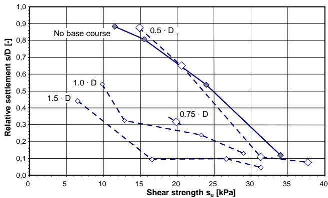
Figure 5 Settlement of the load piston after 100000 cycles, unreinforced systems
