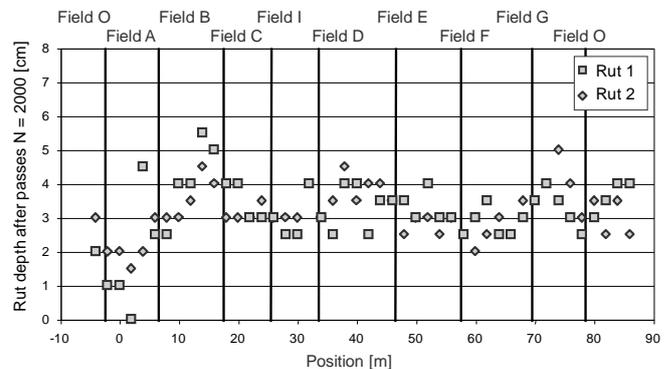
Figure 18 Rut depths after about 2000 passes of loaded trucks
