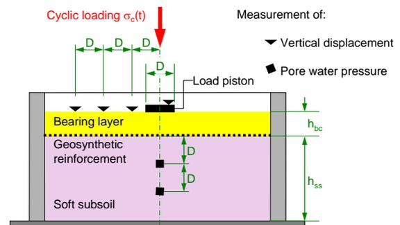
Figure 1 Setup of the model scaled loading tests
