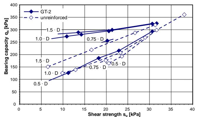
Figure 4 Results of the static loading tests featuring the geosynthetic GT-2
