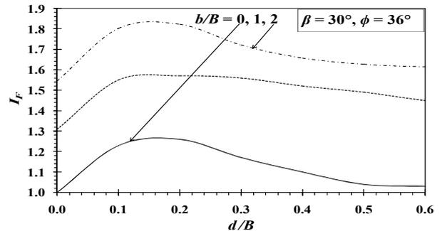
Figure 5 Variation of  $I_F$  with  $d/B$  for  $b/B = 0, 1, \text{ and } 2$
