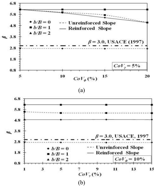
Figure 9 (a) Variation of  $\beta$  with  $CoV_\phi$  of unreinforced and reinforced slopes with  $b/B = 0, 1, \text{ and } 2$ ; (b) Variation of  $\beta$  with  $CoV_\gamma$  of unreinforced and reinforced slopes with  $b/B = 0, 1, \text{ and } 2$
