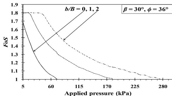
Figure 4 Variation of  $FoS$  with Applied pressure for  $b/B = 0, 1, \text{ and } 2$
