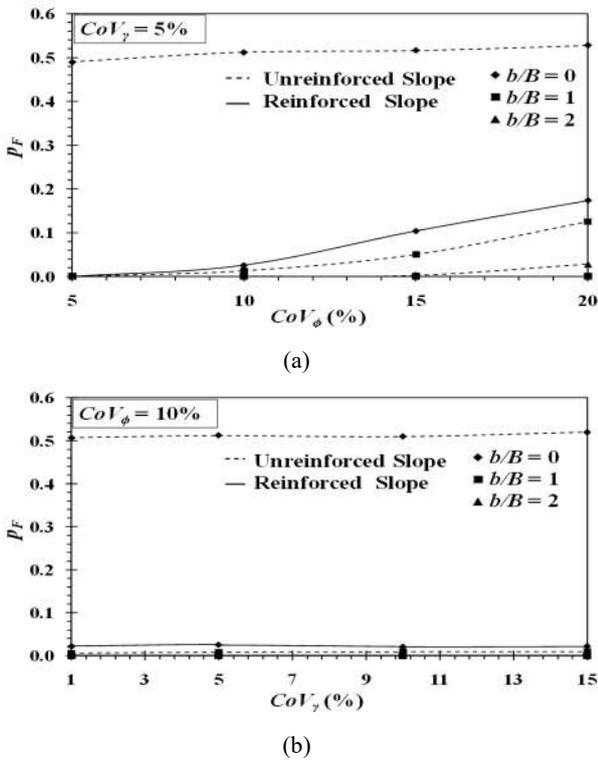
Figure 7 (a) Variation of  $p_F$  with  $CoV_\phi$  of unreinforced and reinforced slopes with  $b/B = 0, 1, \text{ and } 2$ ; (b) Variation of  $p_F$  with  $CoV_\gamma$  of unreinforced and reinforced slopes with  $b/B = 0, 1, \text{ and } 2$
