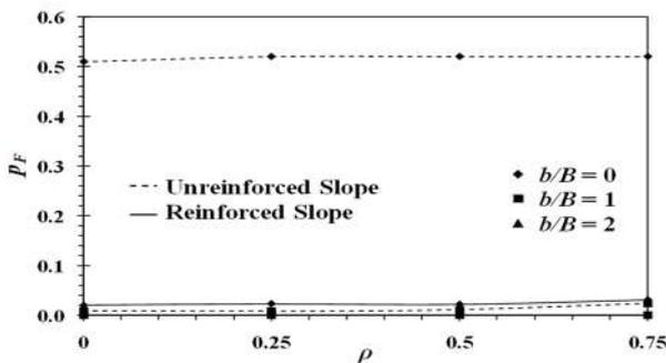
Figure 10 Variation of  $p_F$  with  $\rho$  for unreinforced and reinforced slopes with  $b/B = 0, 1, \text{ and } 2$
