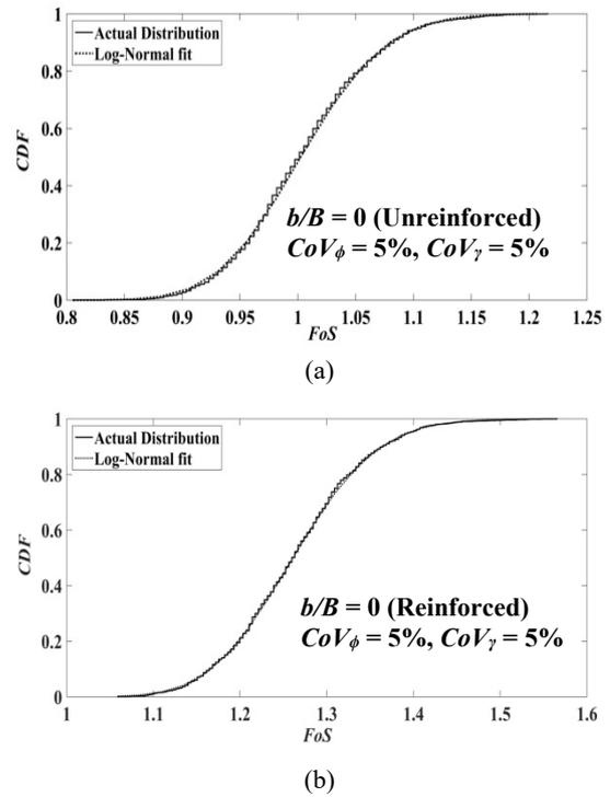
Figure 8 (a) Plot of Actual Distribution of  $FoS$  and Log-Normal fit of  $FoS$  for (a) unreinforced slope and (b) reinforced slope
