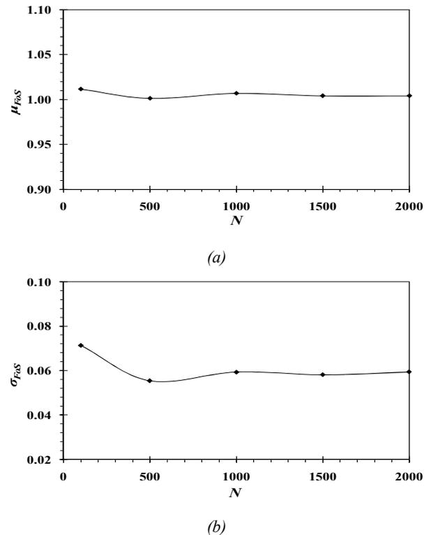
Figure 2 (a) Variation of mean of  $FoS$  with  $N$ ; (b) Variation of standard deviation of  $FoS$  with  $N$
