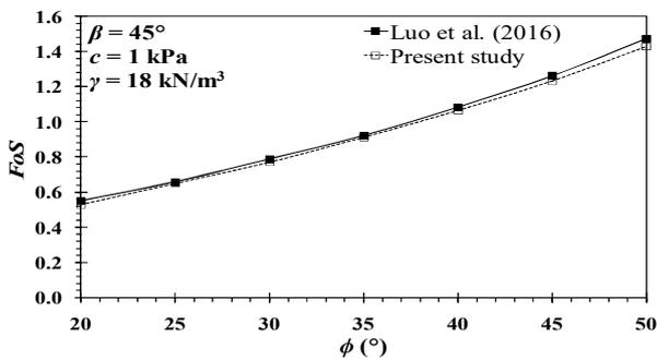
Figure 3 Comparison between the value of  $FoS$  with  $\phi$  obtained from Luo *et al.* (2016) and the present study
