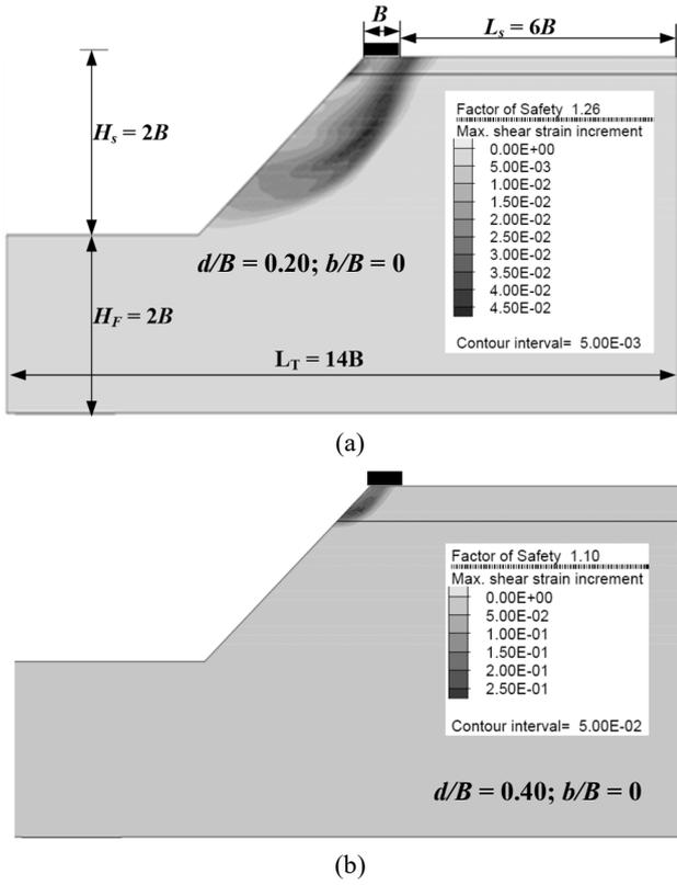
Figure 6 (a) Shear strain increment plot when reinforcement is placed at smaller depth ( $d/B=0.20$ ); (b) Shear strain increment plot when reinforcement is placed at higher depth ( $d/B=0.40$ )
