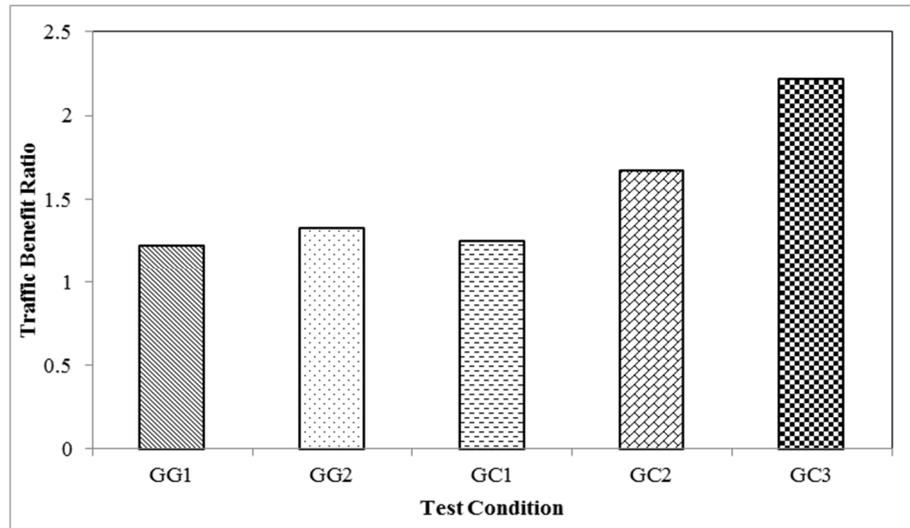
Figure 8 Variation of traffic benefit ratio with the geosynthetic reinforcement
