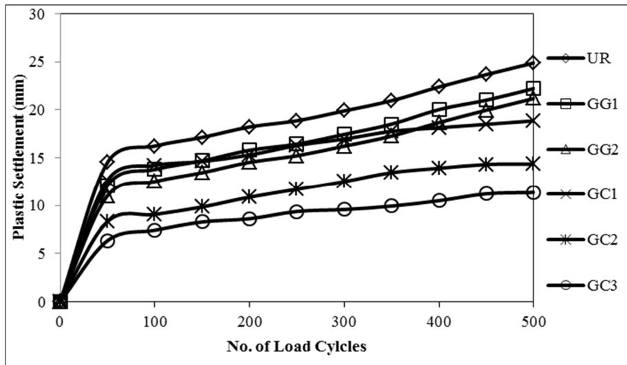
Figure 5 Variation of plastic settlement with number of load cycles in unreinforced and geosynthetic reinforced test sections
