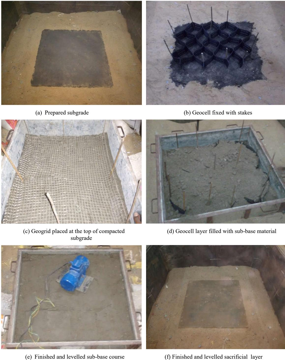
Figure 2 Stage construction for the construction of model pavement sections
