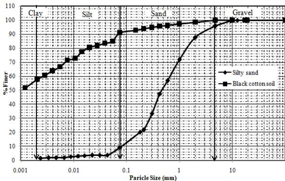
Figure 1 Grain size distribution curves of soils
