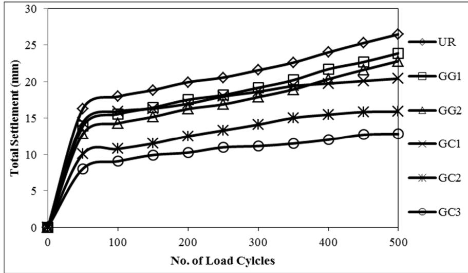
Figure 4 Variation of total settlement with number of load cycles in unreinforced and geosynthetic reinforced test sections
