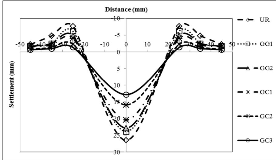
Figure 7 Surface profiles of unreinforced and geosynthetic reinforced model pavement sections at the end of 500 load cycles
