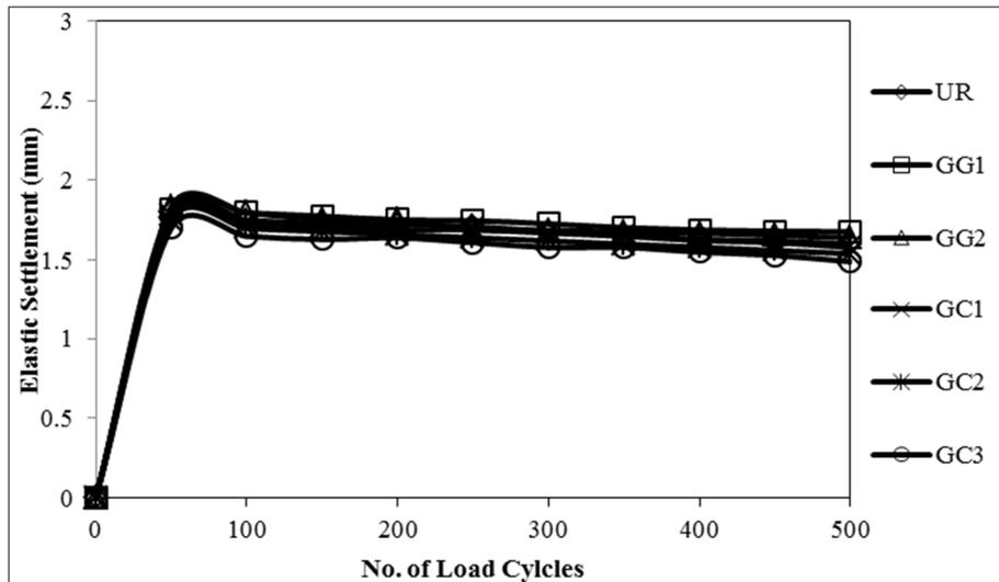
Figure 6 Variation of elastic settlement with number of load cycles in unreinforced and geosynthetic reinforced test sections
