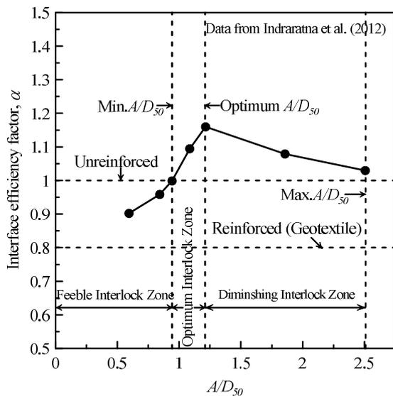
Figure 2 Variation of interface efficiency factor ( $\alpha$ ) with  $A/D_{50}$  (modified after Indraratna et al. 2012)
