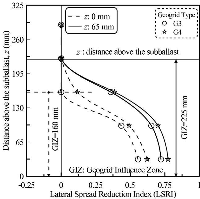
Figure 4 Variation of lateral spread reduction index with distance above the subballast (data sourced from Indraratna et al. 2013)
