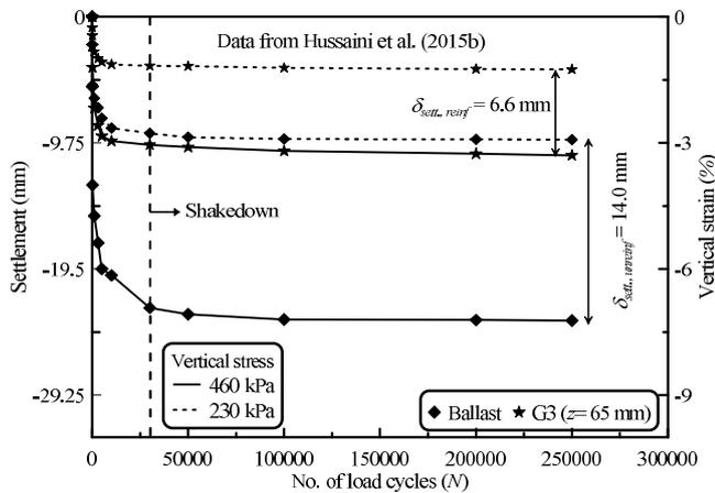
Figure 6 Role of geogrid in reducing the differential settlement in ballast (modified after Hussaini et al. 2015b)
