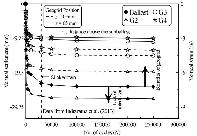
Figure 3 Vertical settlements in unreinforced and geogrid-reinforced ballast (modified after Indraratna et al. 2013)
