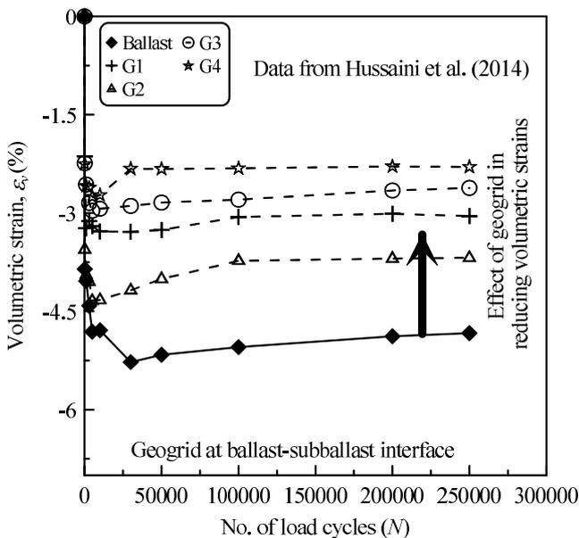
Figure 5 Variation of volumetric strains ( $\epsilon_v$ ) with load cycles ( $N$ ) (modified after Hussaini et al. 2014)
