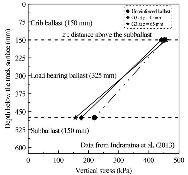
Figure 7 Variation of applied vertical stress with ballast depth (data sourced from Indraratna et al. 2013)
