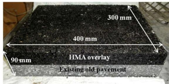
Figure 4 Two layered asphalt slab prepared in the laboratory
