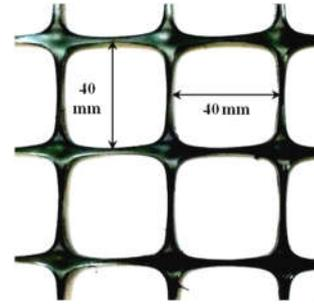
Figure 2 Biaxial polypropylene grid (R2)
