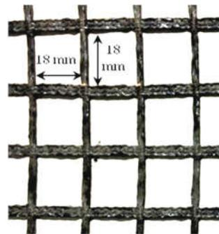
Figure 3 Polyester grid coated with polymer modified bitumen (R3)
