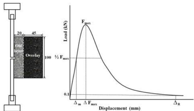
Figure 7 Schematic of Fenix test setup and typical output curve
