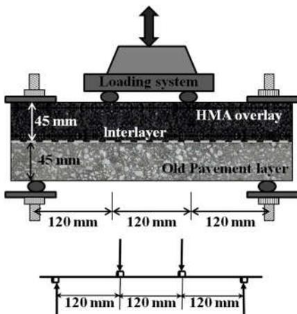
Figure 5 Schematic of flexural fatigue test setup
