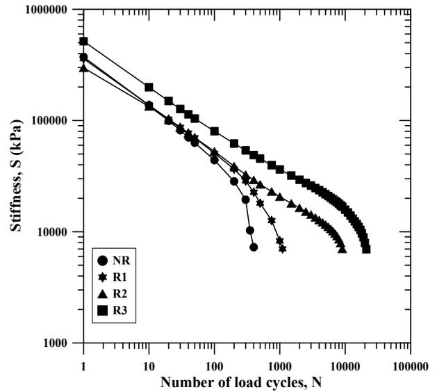
Figure 10 Variation of stiffness with number of load cycles
