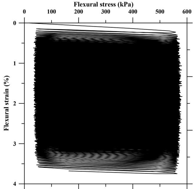
Figure 6 Typical flexural stress-strain plot for control (NR) specimen
