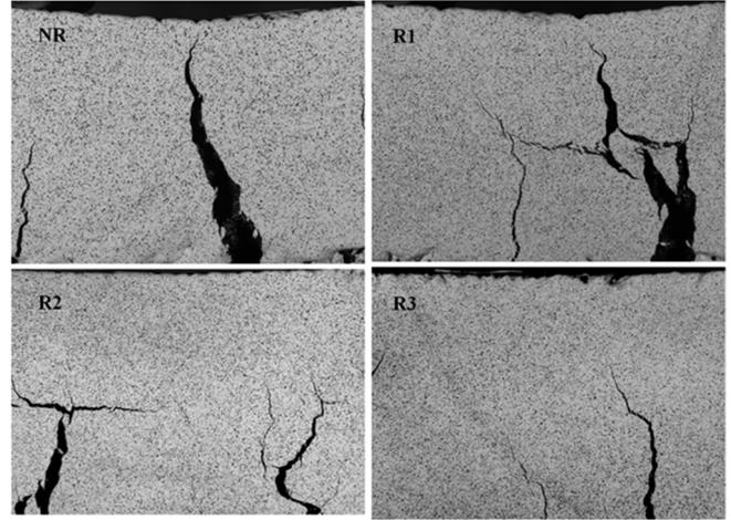
Figure 8 Failure patterns of different two layered asphalt beams
