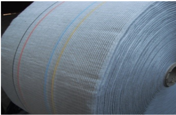
Figure 15 Sensor-enabled geotextile with integrated strain and temperature cables (provided by Dr. Artieres of Tencate Geosynthetics)
