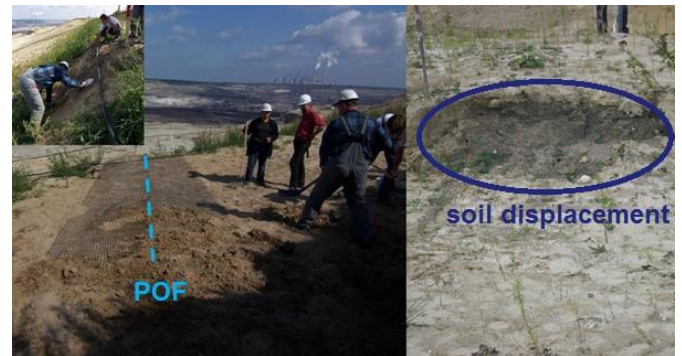
Figure 10 Monitoring of a creeping slope at an open brown coal pit near Belchatow, Poland: Installation of POF-based geogrid (left), Final state after creeping (right)
