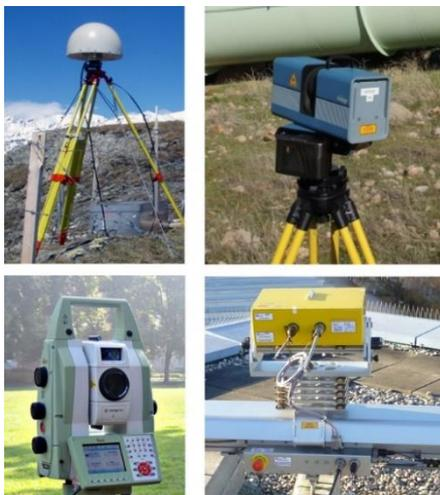
Figure 1 Examples of geodetic instruments: GNSS antenna (top left), laser scanner (top right), total station (bottom left), Ground based interferometric synthetic aperture radar (bottom right)
