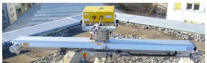
Figure 17 Ground based synthetic aperture radar system moving along a rail
