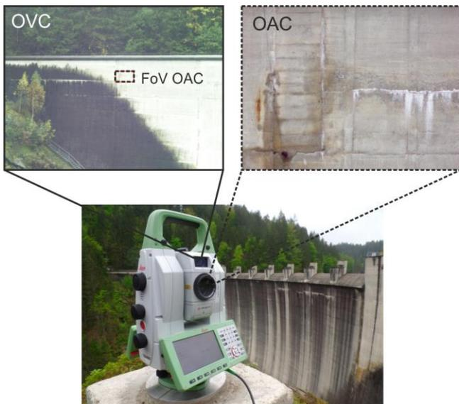
Figure 9 Images of a water dam captured with the cameras integrated in a modern total station
