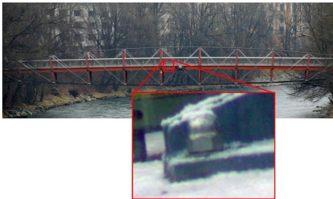
Figure 12 Footbridge and video frame of bolt used for monitoring
