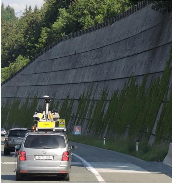
Figure 6 Mobile mapping system mounted on a regular car passing by a typical retaining wall of the Austrian highway
