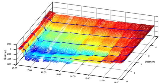
Figure 14 Spatial and temporal strain evolution in extensometer and Brillouin DTSS data
