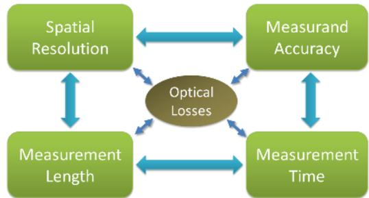
Figure 9 Interdependency of the performance parameters of distributed fiber-optic sensing systems
