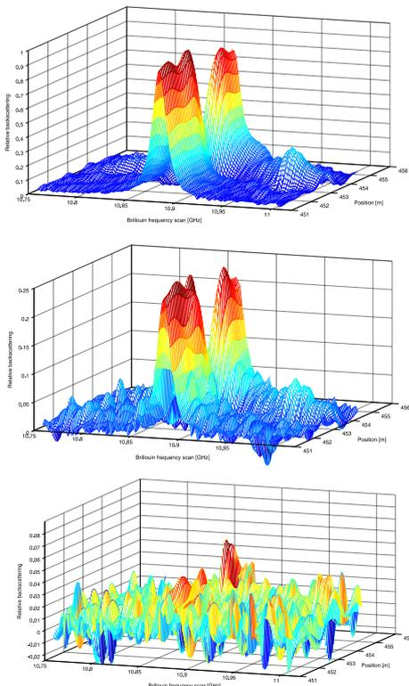
Figure 8 Raw Brillouin data of the measurement traces shown in Figure 7 (Top: 1.4 dB; center: 10 dB; bottom: 19 dB cumulated loss). An unambiguous trace has still be deducted (Figure 7).
