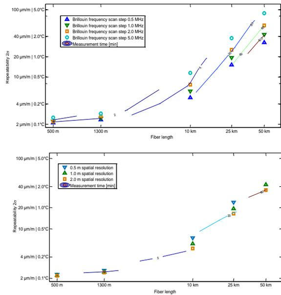
Figure 10 Repeatability and measurement times for a fixed spatial resolution of 1 m (top) and for a fixed Brillouin frequency scanning step of 1 MHz (bottom). The annotated line contours represent the measurement time in minutes
