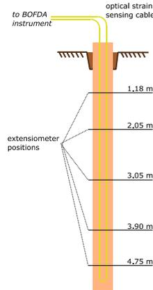
Figure 11 Measurement set-up for static pile load testing
