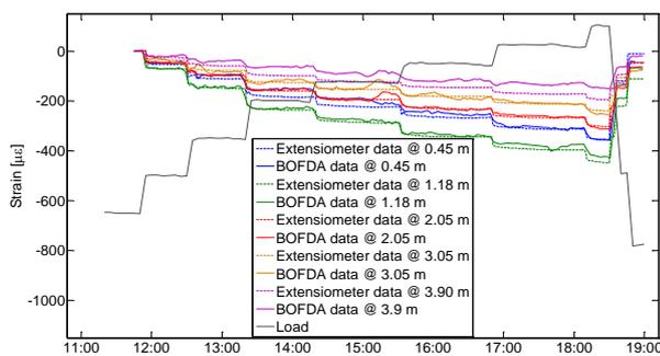
Figure 12 Strain evolution: Extensometer and Brillouin DTSS data
