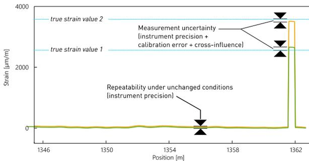
Figure 3 Distributed measurement data illustrating the definitions of uncertainty, accuracy, precision and repeatability
