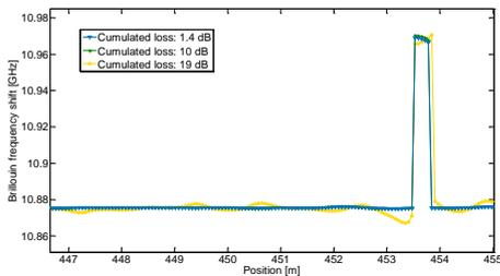
Figure 7 Brillouin DTSS trace of a 0.5 m strained fiber section
