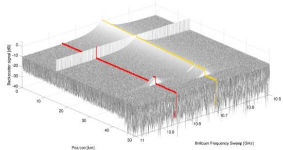
Figure 5 Distributed profile of Brillouin gain from an optical fiber (simulated, as it would be recorded by a Brillouin DTSS system)
