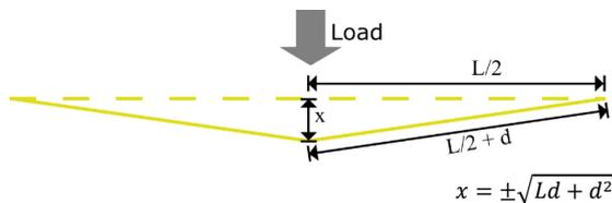
Figure 1 Measured strain based on the length change  $d$  of a distributed sensor over a segment of length  $L$  due to an orthogonal displacement  $x$ . The challenge:  $d$  will be considerably smaller than  $x$
