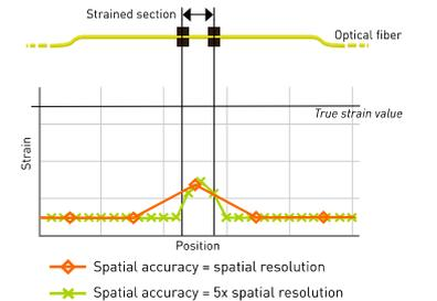
Figure 2 Definitions of spatial resolution and spatial accuracy for distributed strain data in the case of a step-transition strain event
