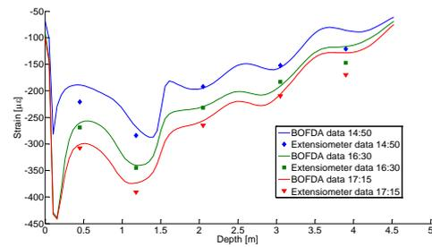
Figure 13 Spatial strain in extensometer and Brillouin DTSS data
