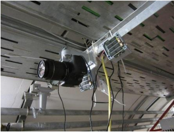
Figure 2 Radiation dosimeters installed in TT10 tunnel
