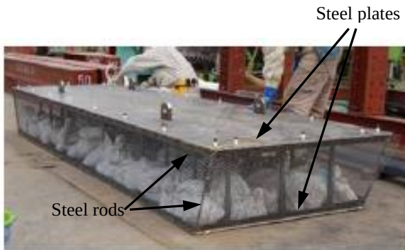
Photo 2 Reduction apparatus of bearing capacity
