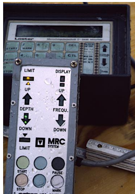
Figure 2 Interactive display that guides the machine operator during the resonance compaction process showing compaction instruction display, Massarsch and Westerberg (1995)
