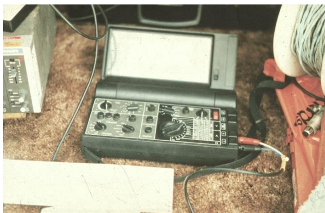
Figure 1 Vibration monitoring of resonance compaction in 1988, at Annacis Island, Canada, (Massarsch and Fellenius 2017)
