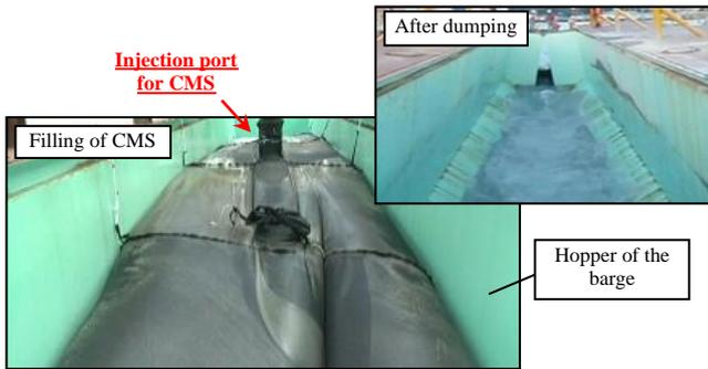
Photo 8 Condition during CMS filling and after dumping
