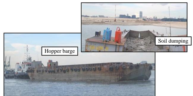
Photo 2 Hopper barge and soil-dumping operation
