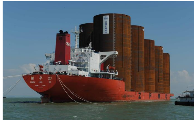
Figure 8 22m diameter pipes for steel cofferdam
