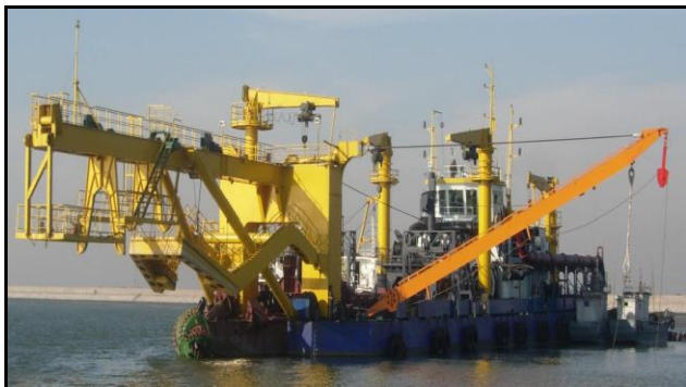
Figure 13 Cutter suction dredger for trench excavation
