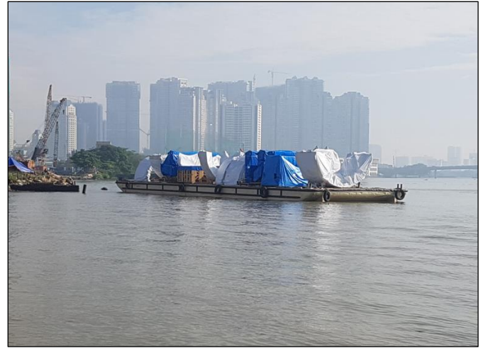
Figure 13 TBM delivery by using barge
