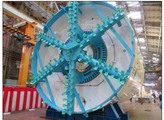
Figure 10 Tunnel Boring Machine (TBM) for CP1b project
