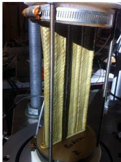
b) Drain being confined after testing
