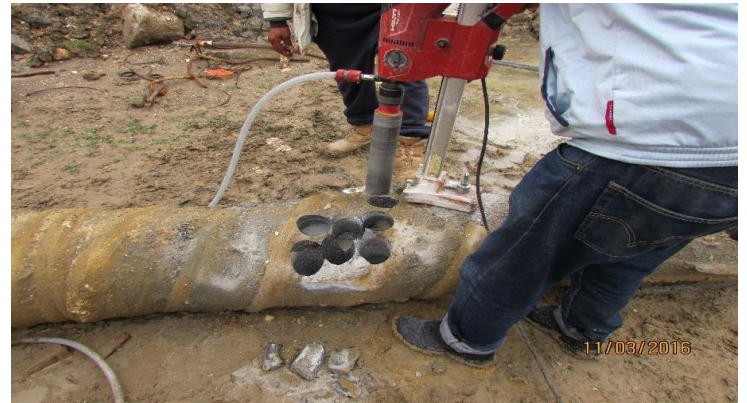
Figure 3 Coring concrete samples from the extracted RIT pile (L = 6 m, D = 0.4 m, Essalema suburb, Tunis City)
