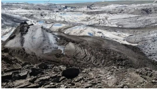
Figure 6 Phosphogypsum deposited with a water content \omega > 30-32\%
