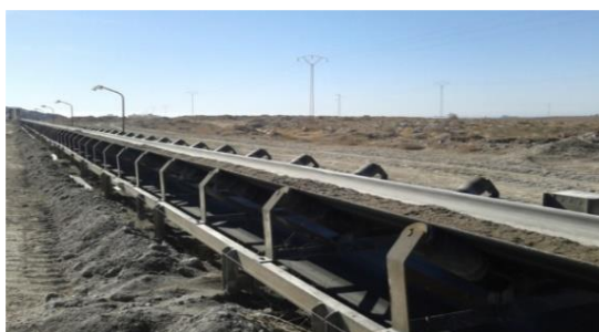
Figure 2 Belt conveyors transporting Phosphogypsum to the deposit site via dry process – The Skhira City Unit
