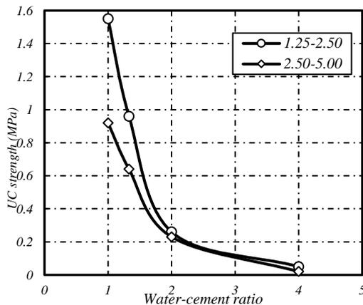
Figure 6 Uniaxial compressive strength with different water-cement ratios after 7 days curing time
