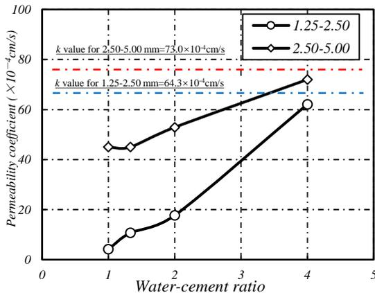
Figure 3 Permeability coefficient versus water-cement ratios after 7 days curing time
