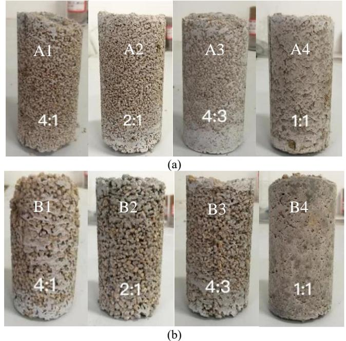
Figure 4 Cement-treated samples after 7 days curing: (a) 1.25-2.50 mm; (b) 2.50-5.00 mm
