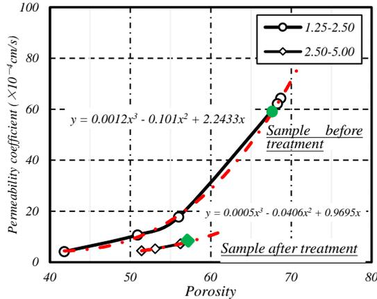
Figure 5 Relationship between permeability coefficient and porosity of test sands
