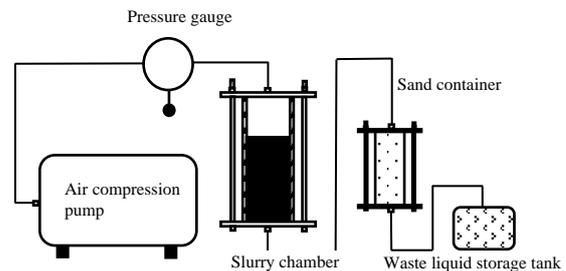
Figure 1 Diagram of grouting system in this study
