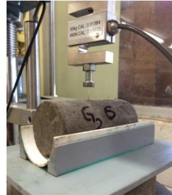
Figure 2 Needle penetration resistance test system
