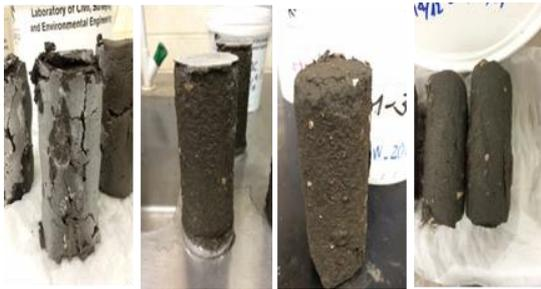
Figure 6 Soil-cement samples exposed to 1000% SW (from left to right: 42, 58, 118 and 208 days)
