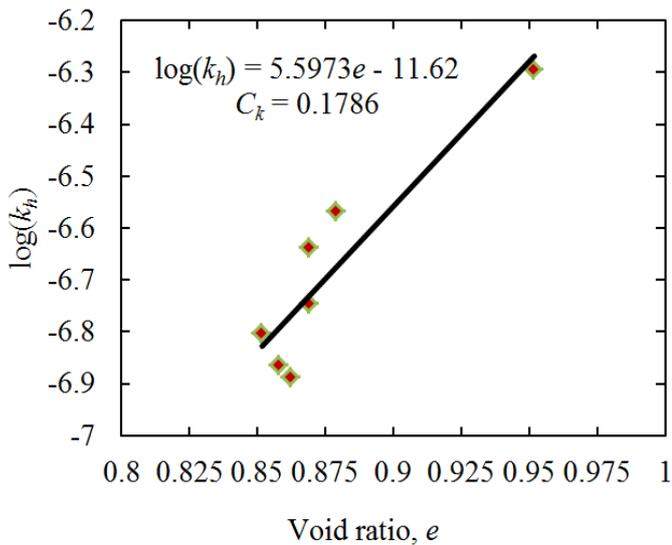
Figure 3 The relationship between void ratio and semi – log horizontal permeability (Vu and Yang, 2016)
