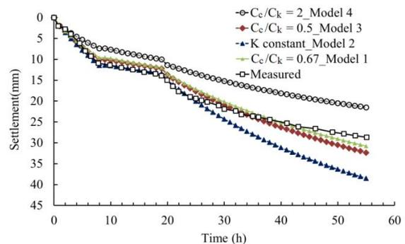
Figure 6 The measured settlement and predicted settlement of all the numerical models
