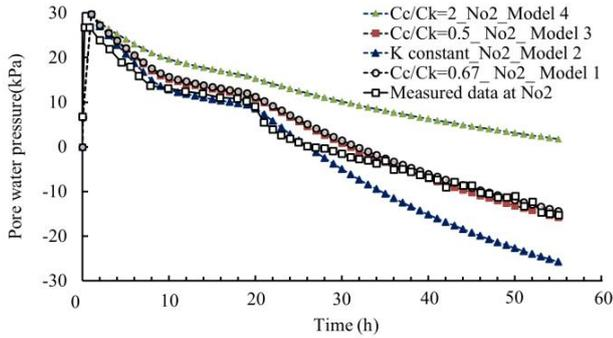
Figure 7 The measured and predicted pore water pressure at the piezometer No2
