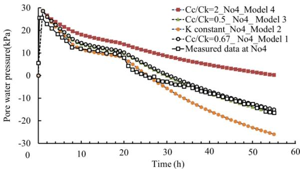
Figure 8 The measured and predicted pore water pressure at the piezometer No4
