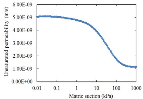
Figure 5 The assumed suction – unsaturated permeability relationship (Vu and Yang, 2016)
