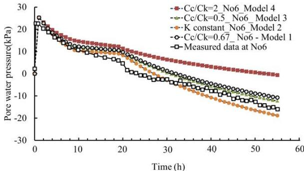
Figure 9 The measured and predicted pore water pressure at the piezometer No6
