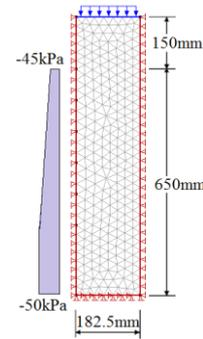
Figure 4 Axisymmetric finite-element mesh
