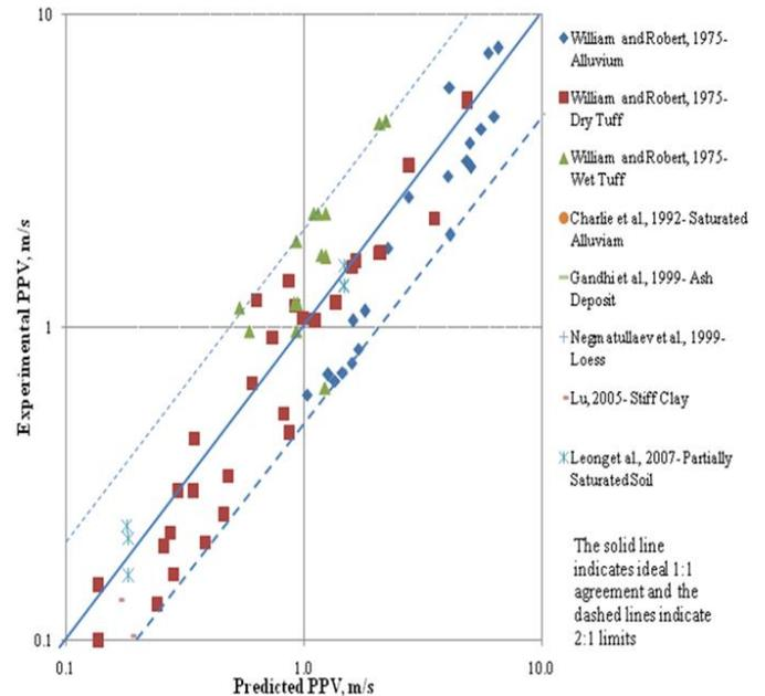
Figure 2 Comparison between experimental PPV and predicted PPV using proposed empirical model in present study
