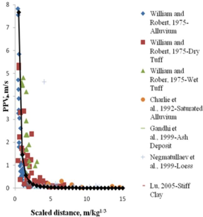
Figure 1 Plot of normalized PPV (m/s) as a function of Scaled distance (m/Kg<sup>1/3</sup>) for experimental data
