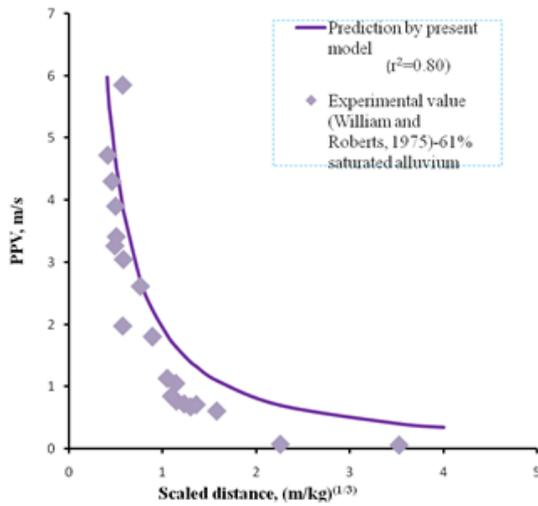
Figure 5 Prediction by present soil model for 61% saturated alluvium experimental values
