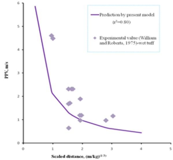
Figure 7 Prediction by present soil model for saturated tuff experimental values
