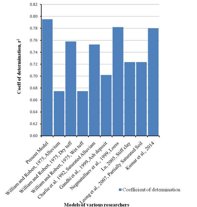
Figure 3 Comparison of Coefficient of determination ( $r_{xy}^2$ ) of empirical models of various researchers
