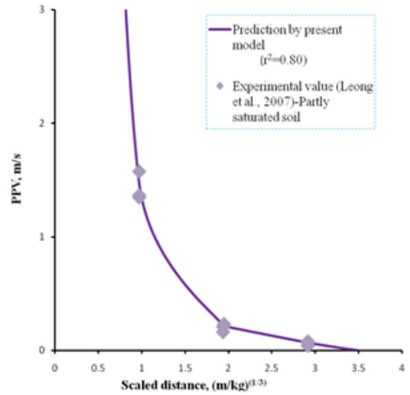
Figure 8 Prediction by present soil model for partly saturated soil experimental values
