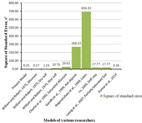
Figure 4 Comparison of square of Standard Error ( $s_{xy}^2$ ) of empirical models for various researchers
