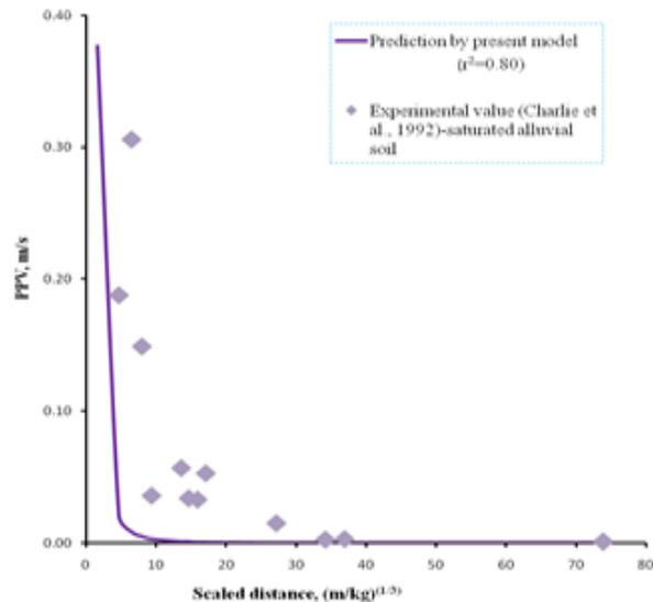
Figure 9 Prediction by present soil model for saturated alluvial soil experimental values
