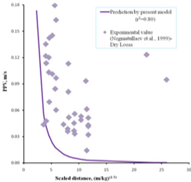
Figure 10 Prediction by present soil model for dry loess experimental values
