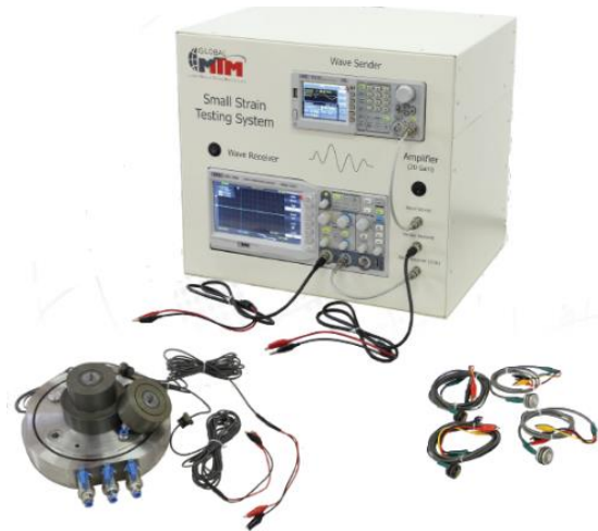
Figure 4 Bender element accessories for small strain wave testings
