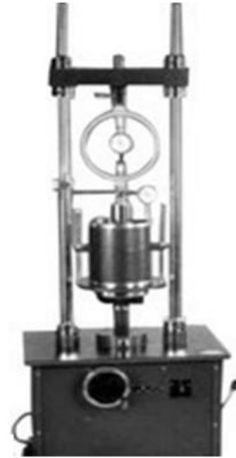
Figure 2 Load Frame used for small scale cyclic load tests
