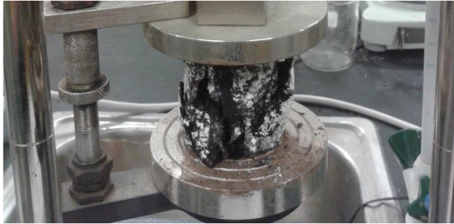
Figure 1 Unconfined Compression Test for Peat Mixed with Peat Ash
