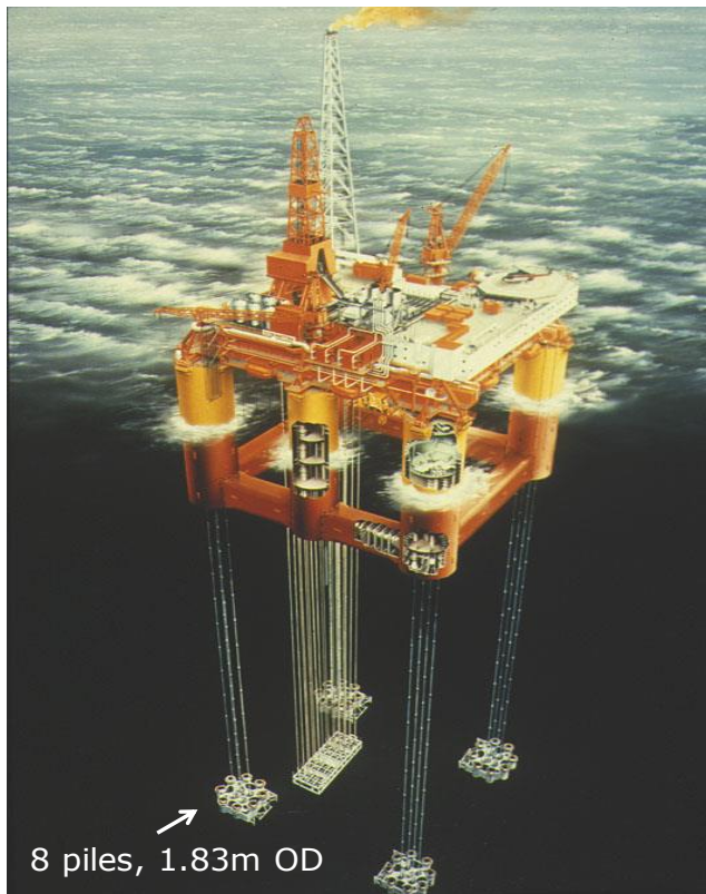
Figure 10 Schematic of Hutton TLP, showing foundation arrangements, after Jardine (1985).
