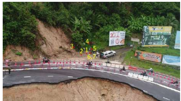
Figure 7 Location of installed sensors; 1: Piezometer (6 m), 2: Tensiometer (2.67 m), 3: Tiltmeter (back slope), 4: Tiltmeter (upper channel), 5: Tiltmeter (water channel), 6: Soil moisture (0.1 m), 7: Soil moisture (0.5 m) and 8: Rain gauge
