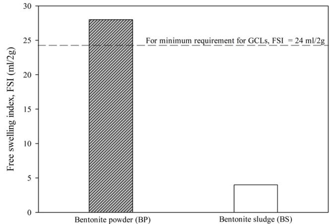
**Figure 3 Results of FSI for BP and BS submerged in deionized water**
