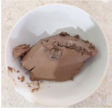
**Figure 1** Bentonite sludge after being treated with polymer
