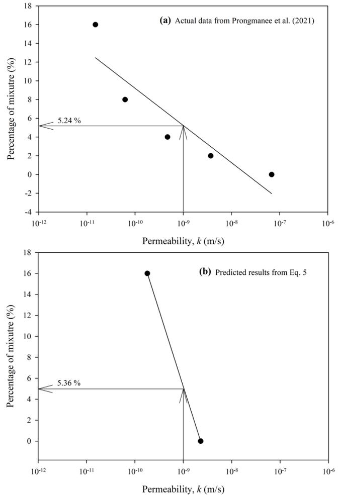
Figure 9 Percentage of mixture versus  $k$  value (a) Actual data and (b) Predicted result
