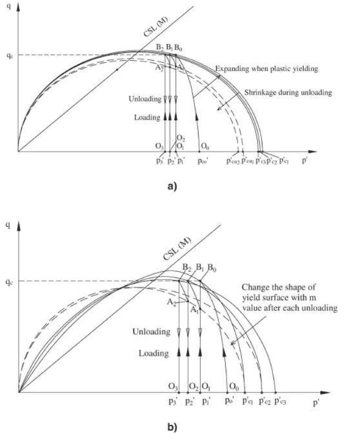
Figure 15 (a) Illustration of Ni et al. (2015) model; (b) Illustration of Truong et al. (2021) model (adopted from Indraratna et al., 2021, with permission from Elsevier)
