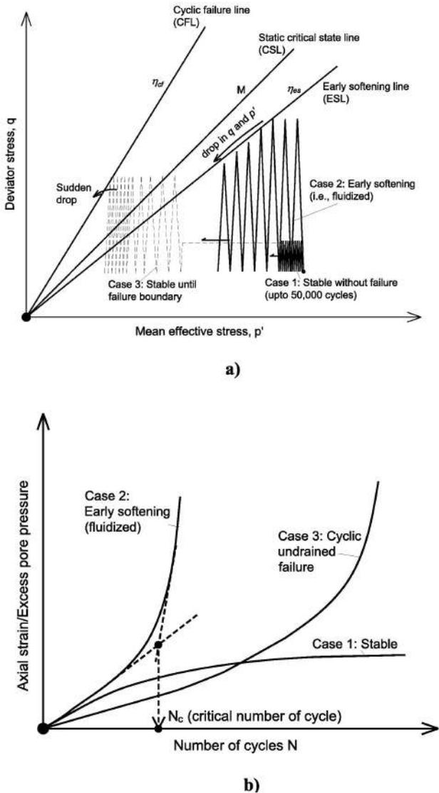
Figure 1 Response of subgrade soil due to cyclic loadings: (a) stress path; (b) axial strain or excess pore water pressure (after Indraratna et al. 2020b, with permission from Elsevier)
