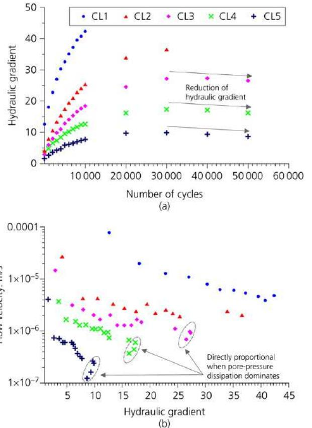
Figure 12 (a) Measured hydraulic gradient during cyclic consolidation test; (b) Relationship between flow rate and hydraulic gradient (after Atapattu et al., 2023, with permission from Emerald Publishing Ltd.)
