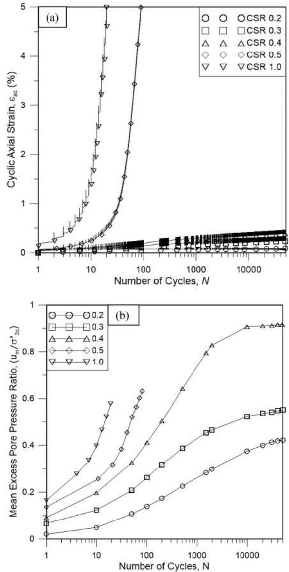
Figure 2 Effect of CSR on axial strains and mean excess pore water pressure ratio (after Indraratna et al. 2020a, with permission from Canadian Science Publishing)
